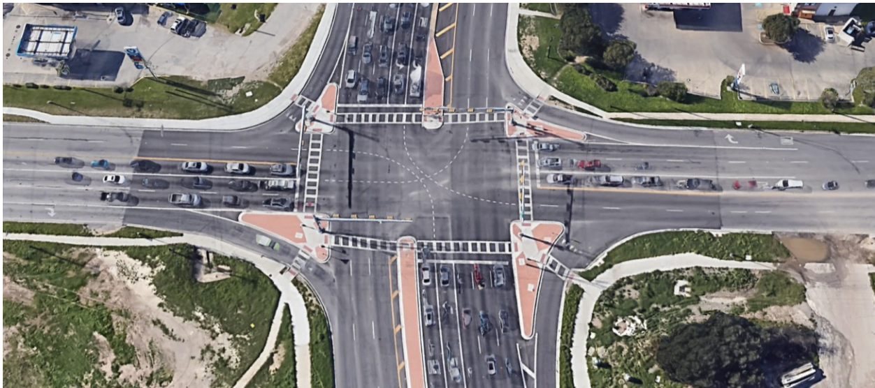
Figure 1. Example a signalized intersection with channelized right turns (CRTs) in Austin, Texas [3].
