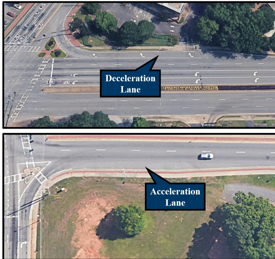
Figure 19. Examples of deceleration and acceleration lanes at CRTs [3].
