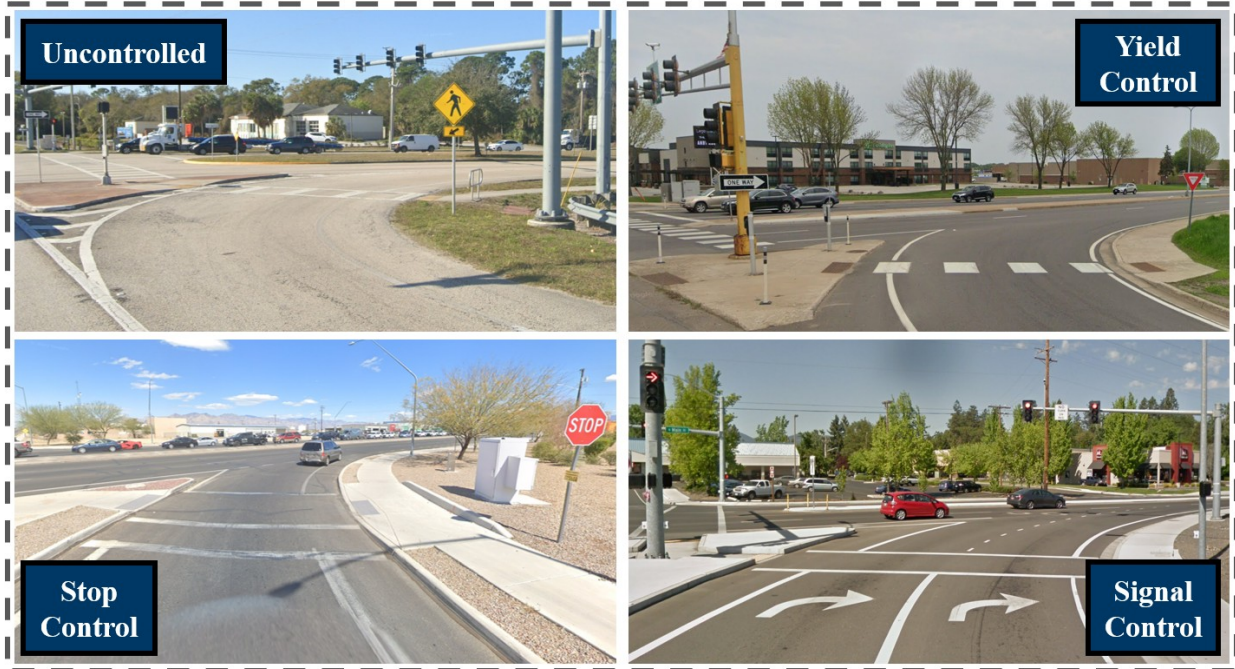
Figure 4. Examples of four common types of vehicular traffic control at CRTs [3].
