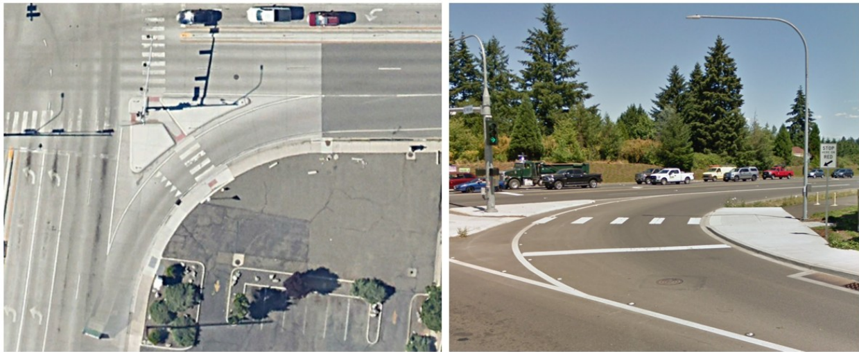
Figure 12. Examples of center-perpendicular crosswalk placement at CRTs [3].
