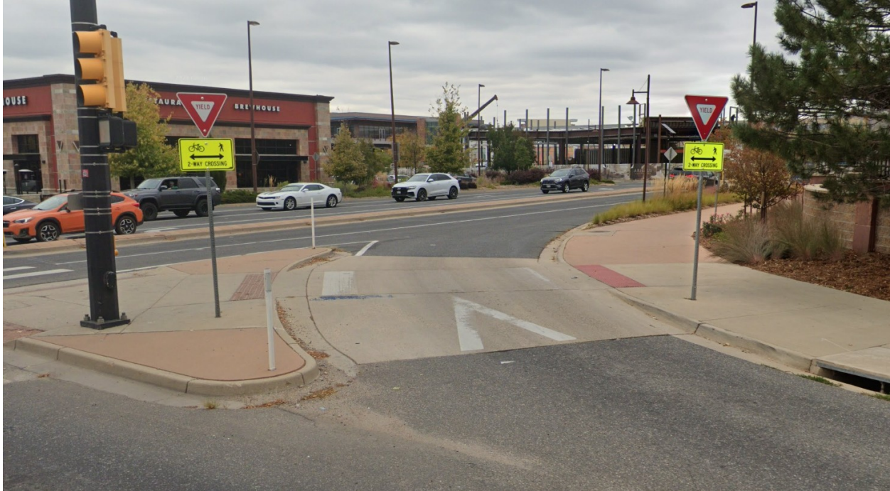
Figure 10. Example of raised crossing at a CRT [3].
